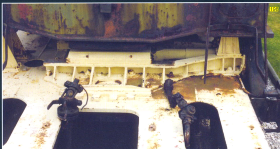
198 199 200 The front of the traversing mechanism. Note the sliding cover for the operating shaft.
