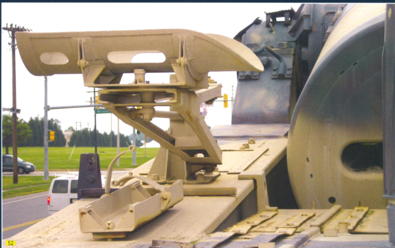
52 A good view of the cartridge catcher. The stand for the rammer should be behind it. This rammer was used to release the breechblock when it became jammed. The container in front is for stowing it (see photo [171]).
