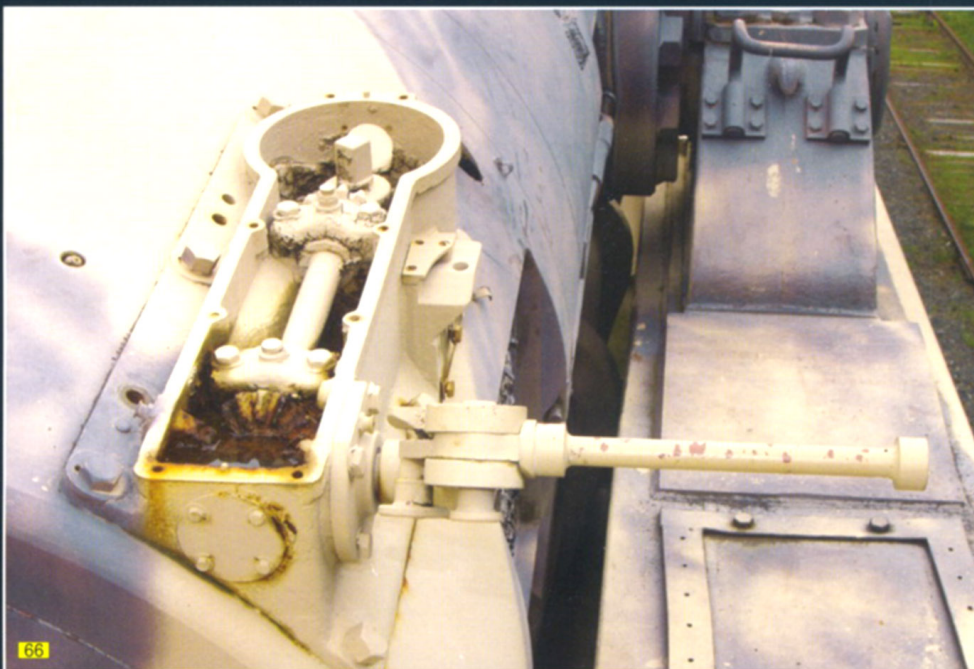
62 63 64 65 66 67 Six different views of the breechblock operating mechanism. It moves the breechblock sideways to open and close the breech. The gears can be clearly seen inside. The cover is missing, as is that on the round hole facing front (see photo [67]). The crank once had a wooden handle.
