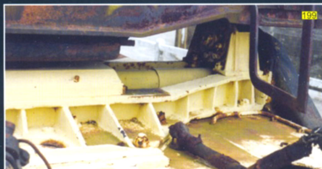
188 190 The side of the front railway truck. This is a twelve-wheel truck, with bogies arranged in two sets of three.
