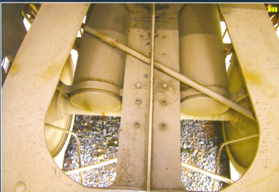
21 22 23 Several views of the pressure vessels for the brakes. The pressure drives central brake cylinders that operate the brakes through a system of rods and hangers.
